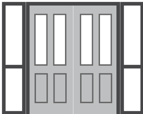
Double Doors with Glazed Sidelights and Midrails
