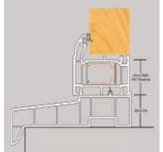
Low Level PVC Frame on Cill
