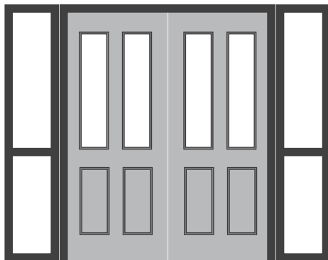
Double Doors with Glazed Sidelights and Midrails
